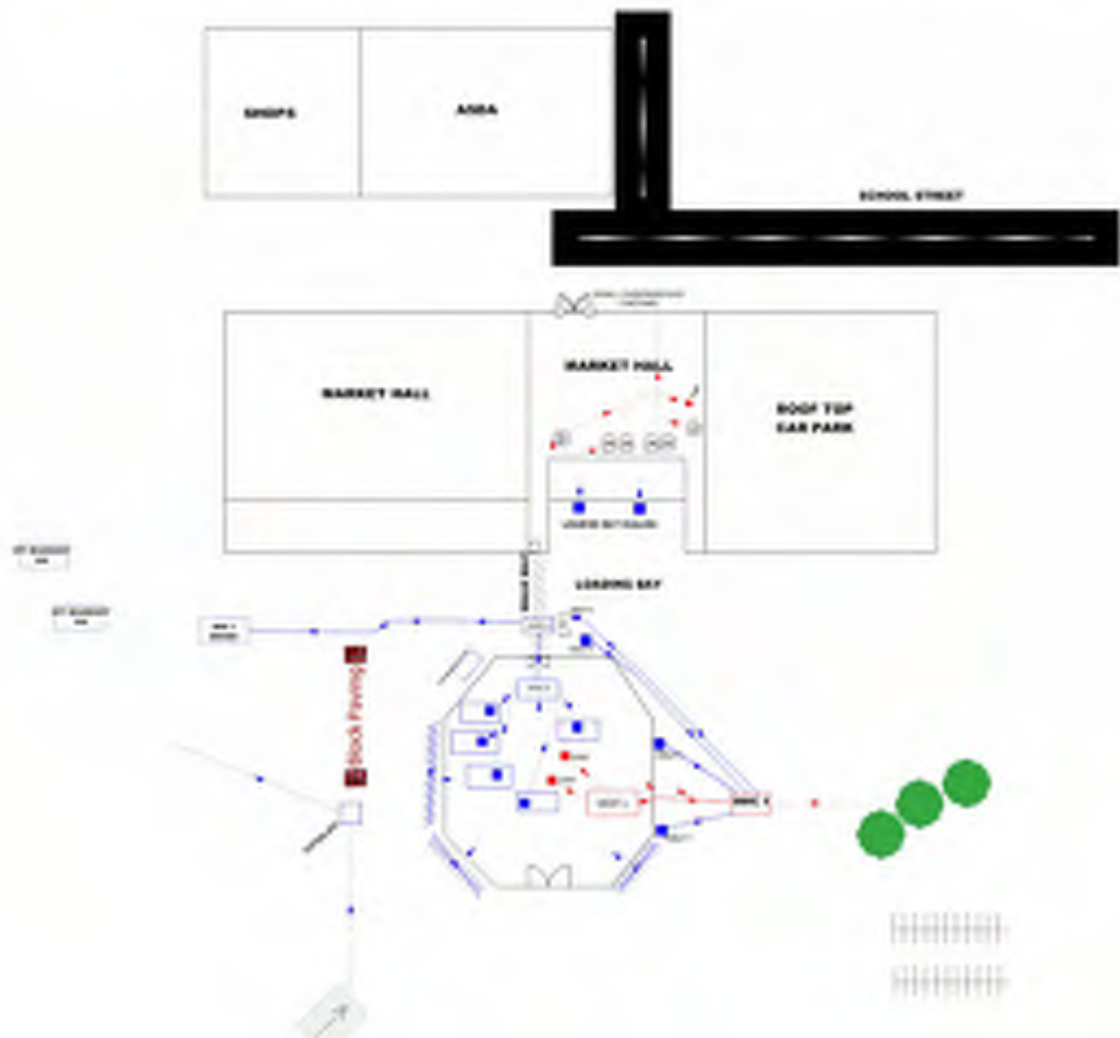
Figure 5: MetroRod CCTV Survey Results Sketch Plan
